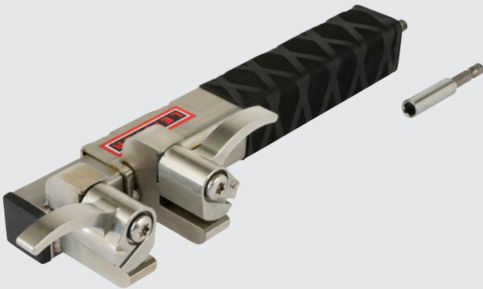
The EXAMO 100 tensile tester tests the weld seam quality of geomembranes. Advantages: tool-free clamping of the specimens, constant tensile speed as well as effortless pulling of the specimens with the cordless screwdriver.
