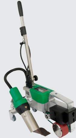
The compact UNIROOF 300 automatic welding machine is ideally suited for welding medium to large flat roofs and is ideal as an entry-level machine due to its simple operation.
