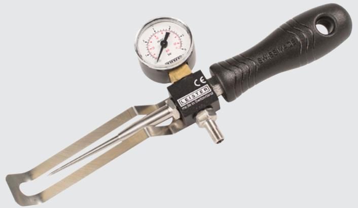
The Leak tester is a reliable compressed air testing device for checking the tightness of overlap seams with test channel. Developed for quality assurance of weld seams in civil engineering, tunnels and landfill sites.
