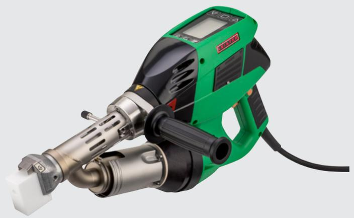
The WELDPLAST S2 TPO extruder is designed specifically for processing thermoplastic elastomers with an olefin base. Thanks to its lightweight size, it is well suited for overhead welding in tunnel construction and underground engineering.
