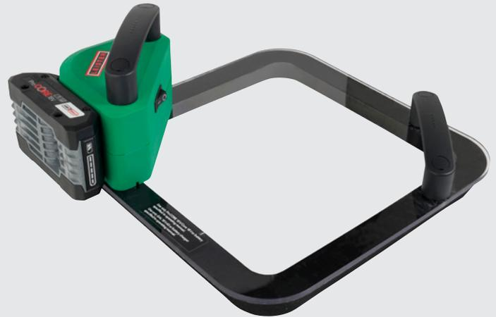
The compact, quiet VACUUM PLATE 100-LP vacuum testing device is designed for leak testing welding seams on roofs and in swimming pools. The integrated AMPShare battery from Bosch enables cordless operation.
